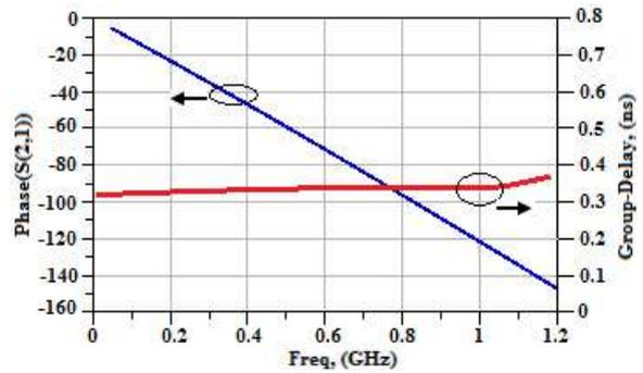
Fig. 7. Phase and group delay for the proposed LPF in the passband
