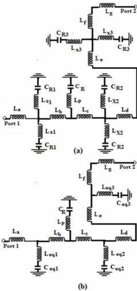
Fig. 6. (a)The LC equivalent circuit of the proposed LPF, and (b) the simplified LC equivalent circuit of the proposed LPF
