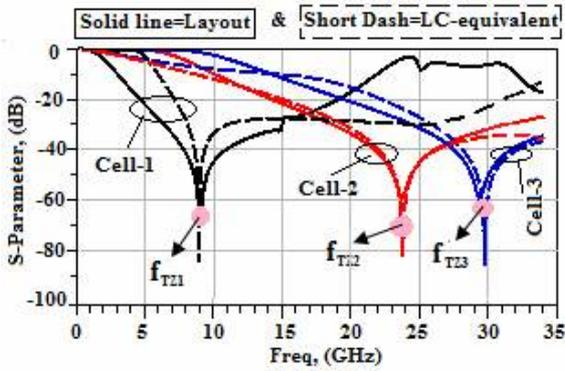
Fig. 3. Simulations (LC and EM) of three suppressor cells
