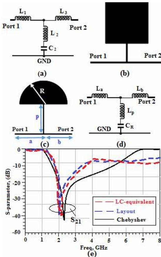
Fig. 1. Resonator, (a) third-order Chebyshev, (b) layout, (c) proposed resonator, (d) LC equivalent circuit and (e) simulations results
