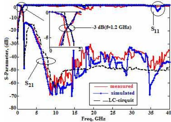
Fig. 5. Simulated, measured and LC equivalent circuit results of the proposed filter
