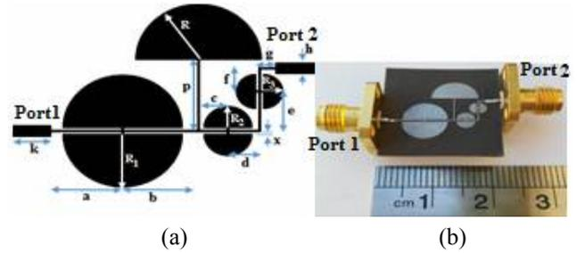
Fig. 4. The proposed LPF (a) layout, and (b) fabricated.
