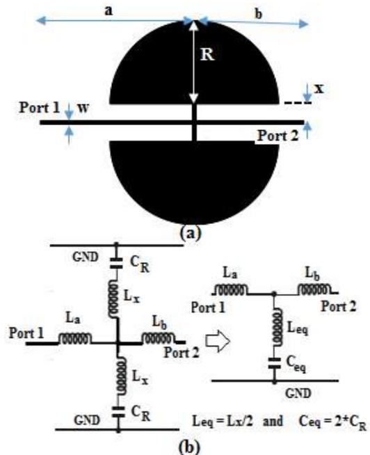
Fig. 2. Suppression cell, (a) layout and (b) LC equivalent circuit
