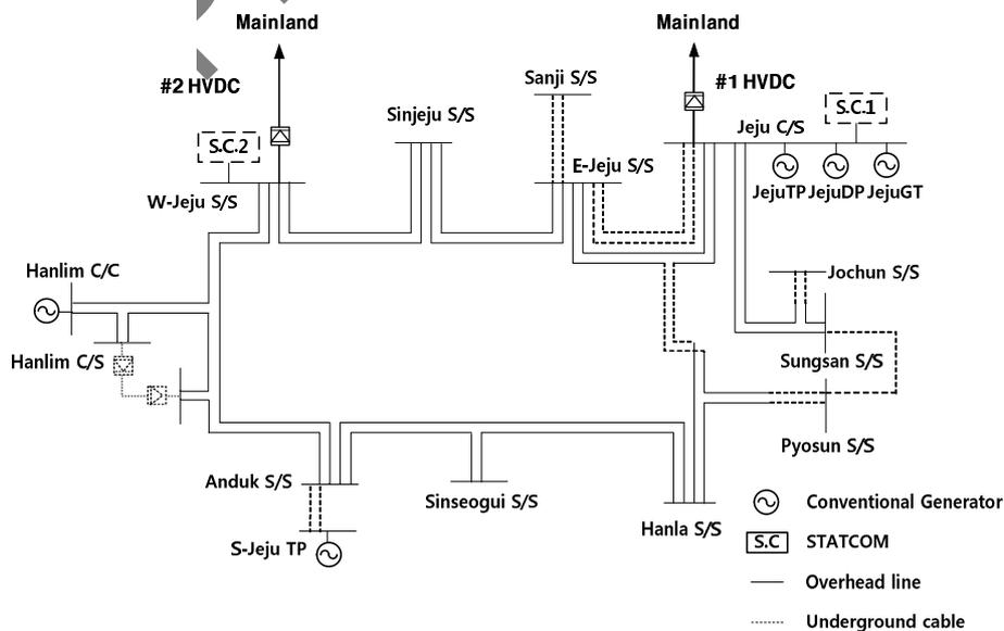
**Fig. 7.** Jeju island power system schematics
