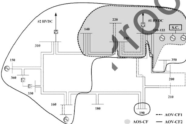
Fig. 10. AOS-CF with #1 shunt compensator installation
