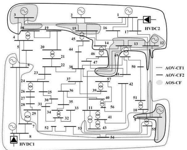
Fig. 6. AOS-CF considering two HVDC converter station
