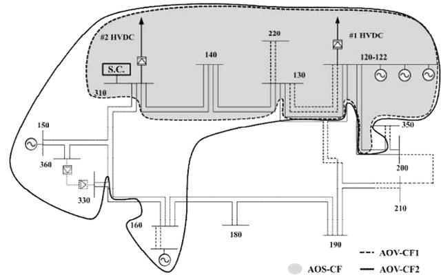
Fig. 11. AOS-CF with #2 shunt compensator installation
