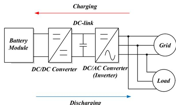
Fig. 1. The general configuration of energy storage system
