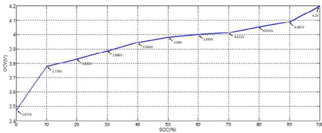
**Fig. 11.** OCV measurement corresponding to the SOC
