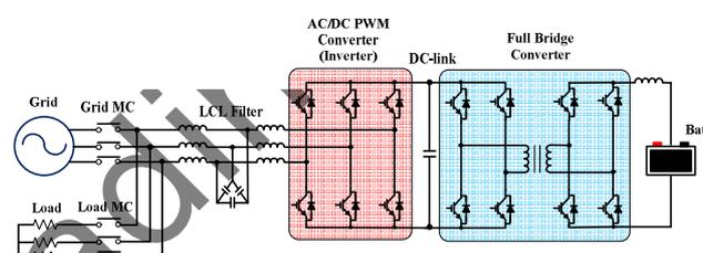
Fig. 2. The configuration of Grid-tied Energy storage system
