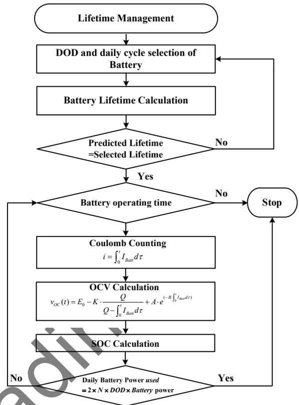
**Fig. 12.** Flow diagram of proposed lifetime management
