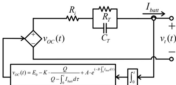
Fig. 9. Battery model coupled with Shepherd and Thevenin model
