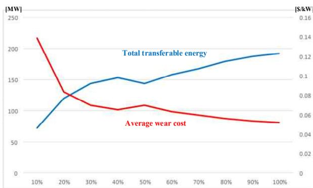
Fig. 6. Average wear cost corresponding to the DOD
