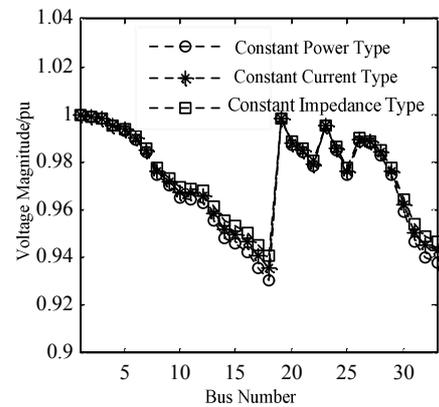
Fig. 7. Node voltage distribution with weakly meshed distribution network
