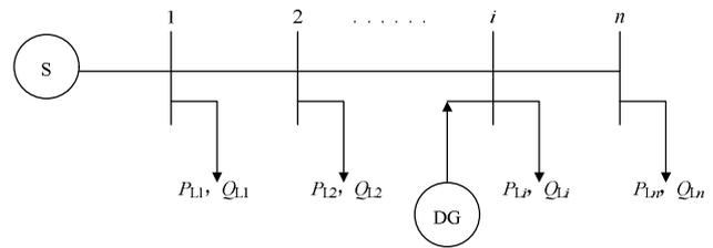
Fig. 1. Single radiant circuit with a DG
