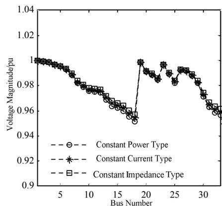
Fig. 11. Node voltage with PV-type DG
