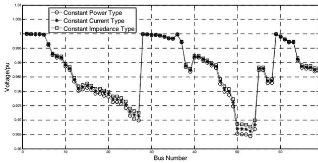
Fig. 15. Node voltage with PI-type DG
