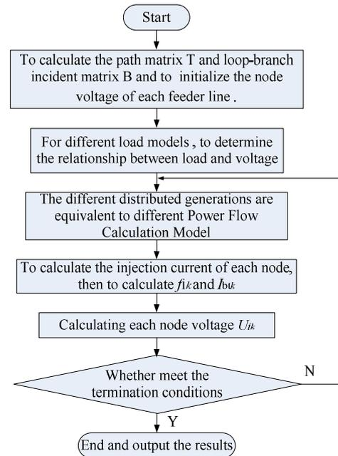
Fig. 5. Power flow algorithm flow chart
