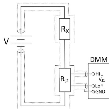
Fig. 3 (a) Voltage source-voltmeter method Dotted lines mean electric shielding
