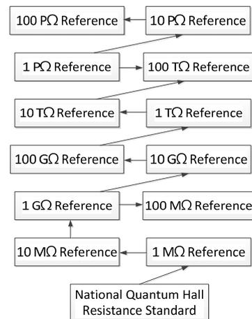
(a) Bridge methods. the 10 to 1 ratio measurements are made for all the comparison.
