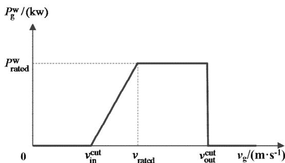
Fig. 1. Relationship between wind turbine output and wind speed
