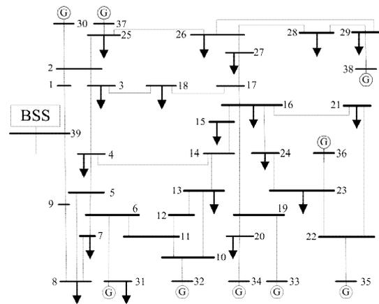
Fig. 7. Modified schematics of IEEE 39-bus system
