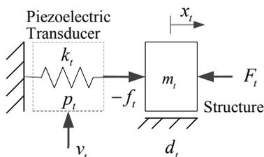
Fig. 1. Ultrasonic transmitter model
