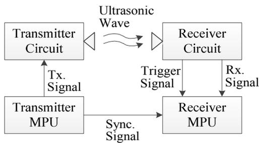
Fig. 7. Experimental setup
