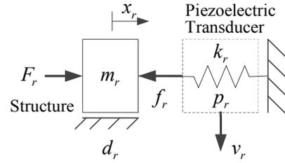
Fig. 2. Ultrasonic receiver model
