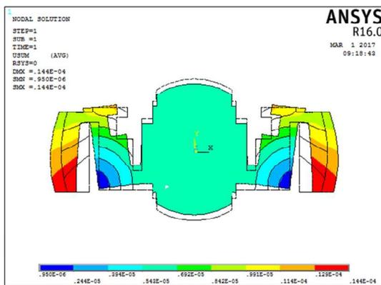
Fig. 7. FEM centrifugal deformation of MSSG rotor
