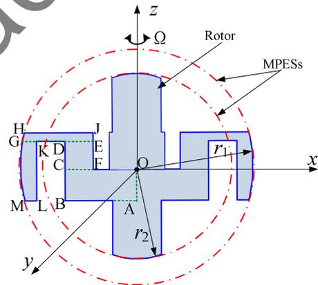
Fig. 3. Computing method of rotor centrifugal deformation radially
