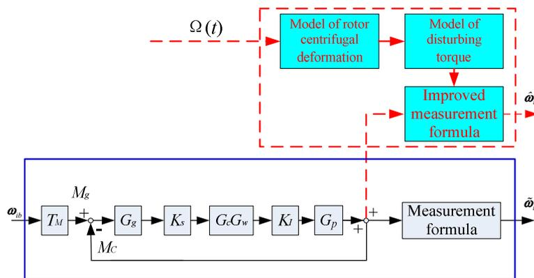
**Fig. 6.** Schematic diagram of the error compensation method
