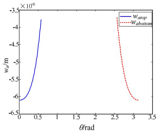
Fig. 4. Centrifugal deformations of the MSSG rotor axially
